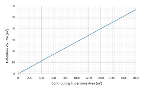
Figure 7: Detention Tank selection chart - Industrial Zones
