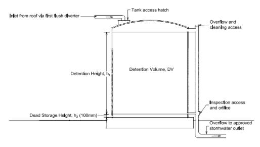
Figure 4: Schematic of Detention Tank configuration
