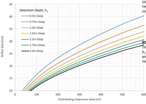
Figure 6: Orifice Sizing Chart (100% impervious area connected to tank)
