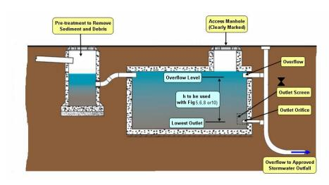
Figure 2: Below ground Detention Tank - typical components
