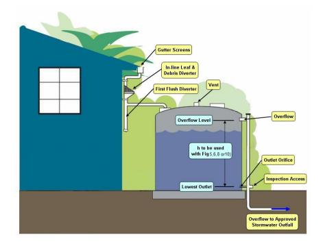
Figure 1: Above ground Detention Tank - typical components
