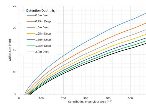
Figure 5: Orifice Sizing Chart (85-95% impervious area connected to tank)
