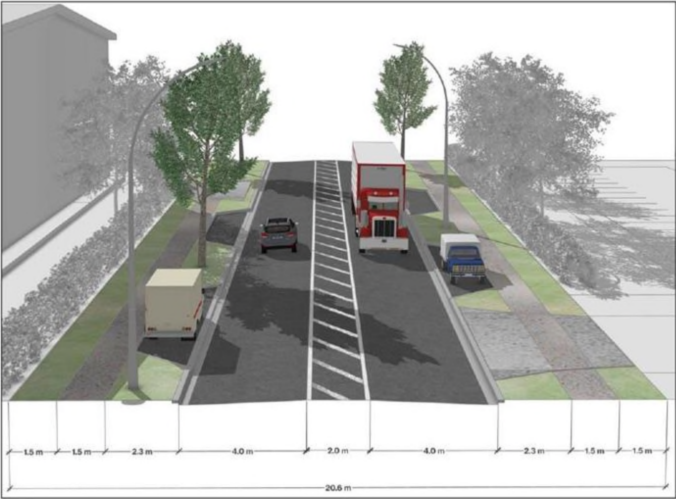
Figure 3.9.2.5.d: Indicative Typical Cross-Section for Local Roads
