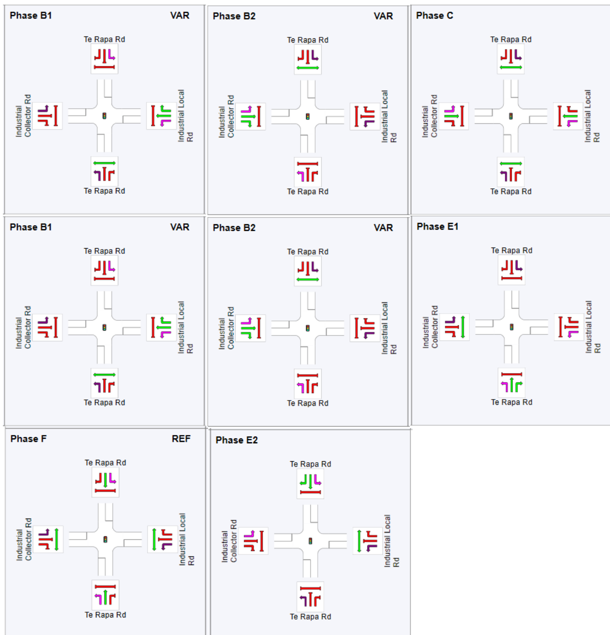
Figure 8: Proposed Phase Sequence – Te Rapa Rd / Access 2 Intersection
