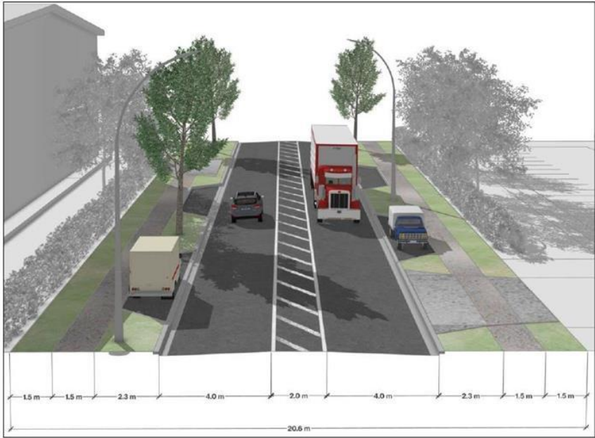
Figure 3.9.2.5.d: Indicative Typical Cross-Section for Local Roads
