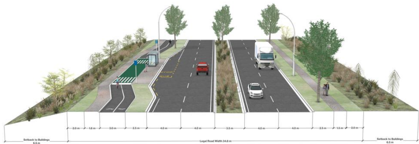
Figure 3.9.2.5.b: Indicative Typical Cross Section of the ultimate Northern River Crossing (Arterial), following upgrade of East-West Road
