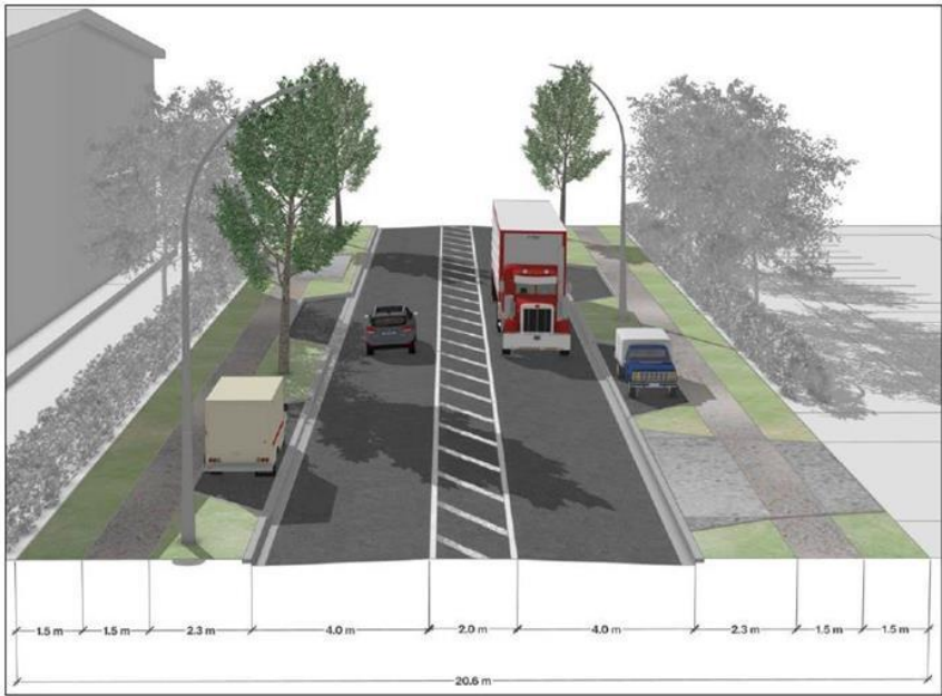
Figure 3.9.2.5.d: Indicative Typical Cross-Section for Local Roads
