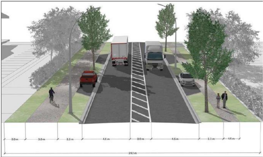
Figure 3.9.2.5.c: Indicative Typical Cross-Section of the Te Rapa Structure Plan Spine Road (Collector)
