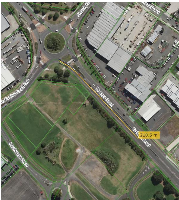
Figure 50: 95 th Percentile Back of Queue on Te Rapa Rd (AM Peak Hour – Infrastructure Scenario 1)
