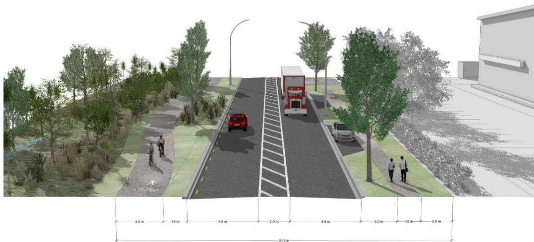
Fig. 19. Proposed typical cross section for the Collector Road, showing the alignment adjacent to the Te Rapa Stream Riparian and Stormwater Reserve.
