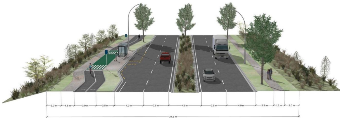
Fig. 18. Proposed Arterial Road typical cross section (East-West Arterial)
