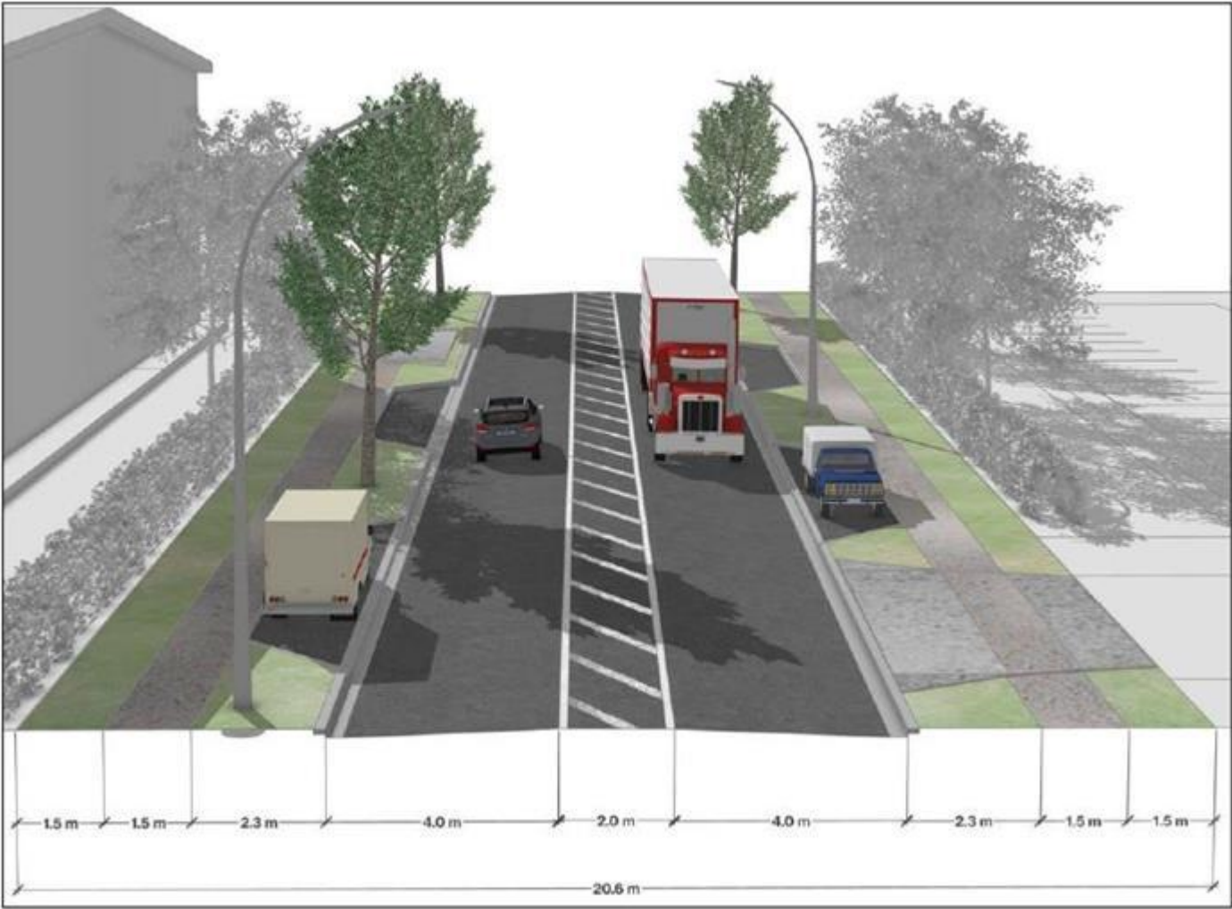
Figure 3.9.2.5.d: Indicative Typical Cross-Section for Local Roads
