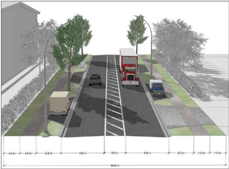
Figure 3.9.2.5.d: Indicative Typical Cross-Section for Local Roads
