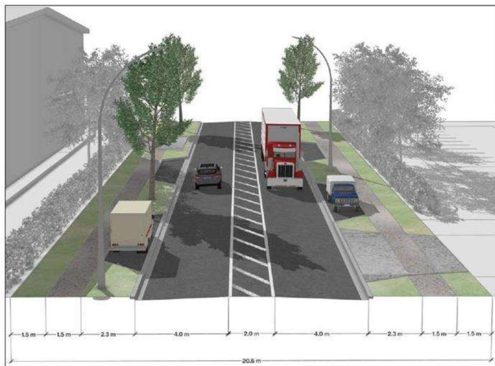
Figure 3.9.2.5.d: Indicative Typical Cross-Section for Local Roads
